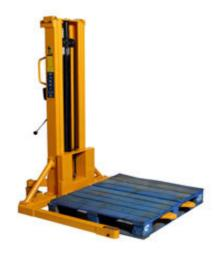
The new GT range addresses the issue of "Full Perimeter Board / CHEP" pallets. The 1225mm inside straddle allows picking of the pallet against the widest side. Available in two models normally ex stock.
